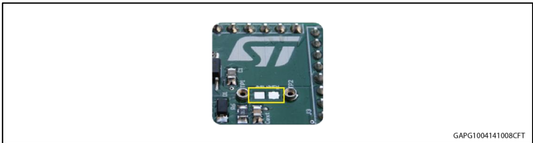
Figure 5: Pads for soldering SMD resistor
